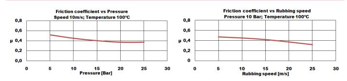
Rubbing speed, temperature and pressure are related. Changing any values will change other. The values shown represent typical conditions, but are not ultimate limits of the material.
